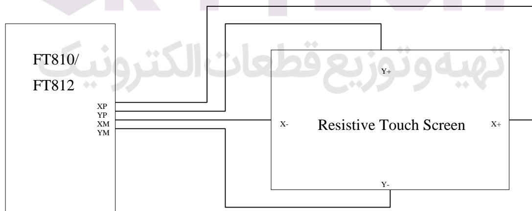
Figure 4-8 Resistive Touch screen connection
